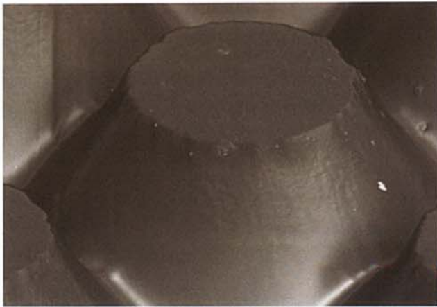
IMAGE 5 A SINGLE DOT, AT 250X SHOWS THE FLAT-TOPPED DOT PROFILE, SHARP BEVEL, AND RELIEF DEPTH AVAILABLE WITH THIS PATENTPENDING DIGITAL PLATE TECHNOLOGY.
